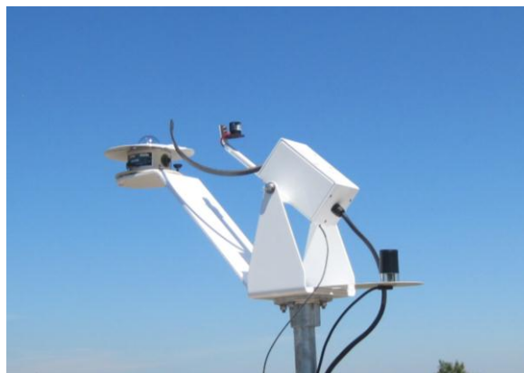
Fig. 2: NEO Primary DAS, Rotating Shadowband Radiometer (RSR2) with Eppley Precision Spectral Pyranometer.
