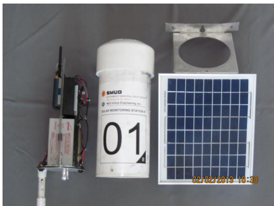
Fig. 4: NEO Secondary DAS, exploded view.
