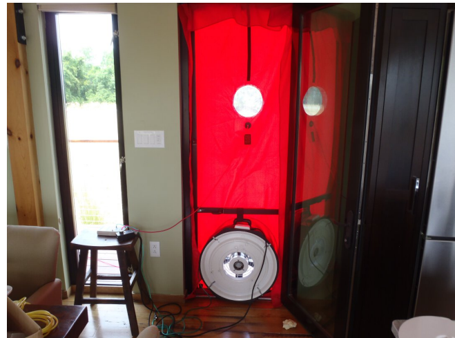
Fig. 3: Photo of the blower door test device installed in a doorway.
