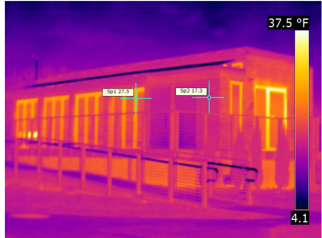
Fig. 2: Thermal imaging of the outside of the building, showing heat loss through door and window frames.
