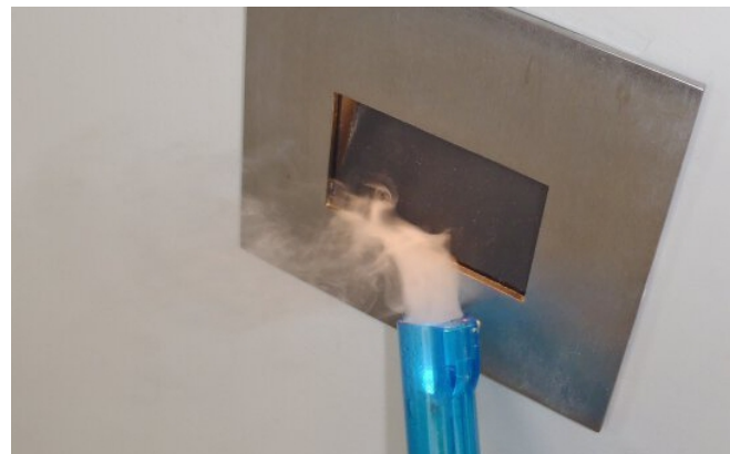
Fig. 4: Photo of smoke testing revealing infiltration.
