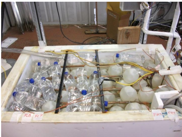
Fig. 1: Prototype thermal storage tank and components.
