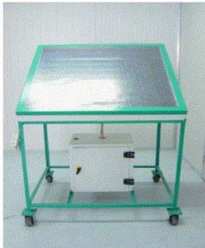
Fig. 1:Solar-powered icemaker without valves [ 12].
