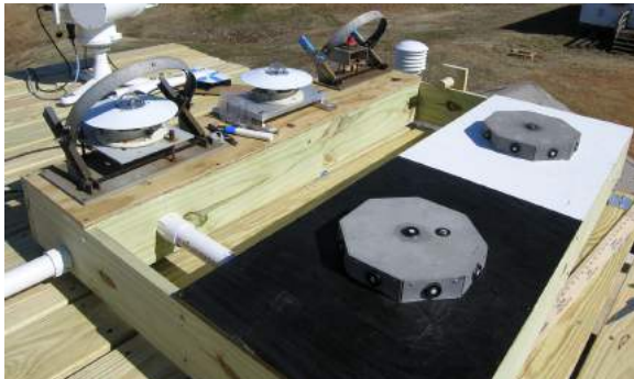
Figure 1: Photocell and irradiance sensors
