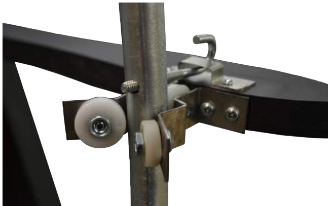
Fig. 8: Rollers connecting metal ring to carriage and pin indicating time of day.
