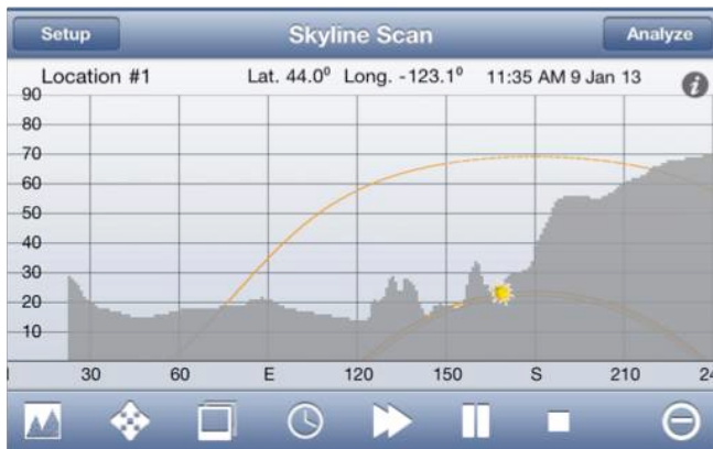
Fig. 7: Unwrapped skyline photo taken in Eugene, Oregon from Solmetric iPV application (screenshot from iPhone)
