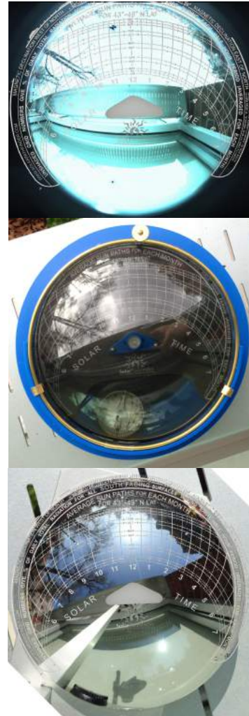
Fig 9. From top, sun path chart from the SunEye, Solar Pathfinder, and HORICatcher for the case study window showing a decrease in truncation of the sky from top to bottom device
