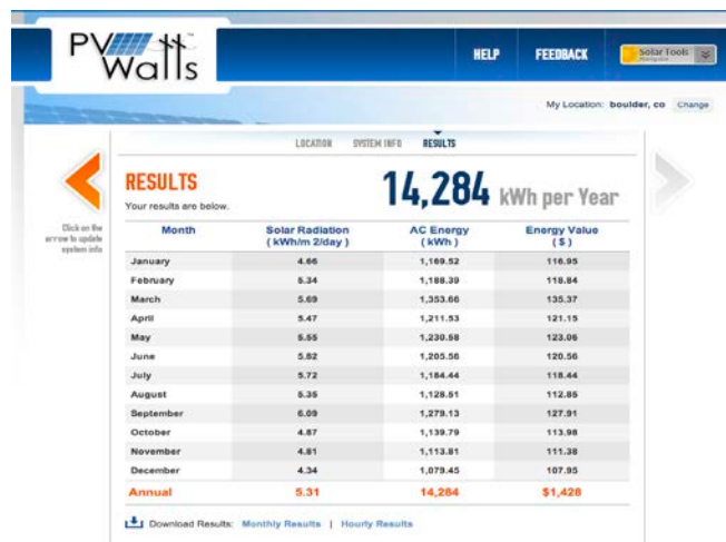
Fig. 5: Spring 2013 release of the PVWatts calculator interface showing the modeled monthly production estimates of a 10-kW PV system in Boulder, CO.
