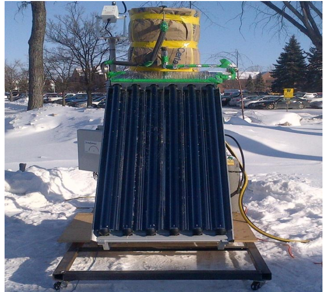
Fig. 4: Front view of the solar water heater.
