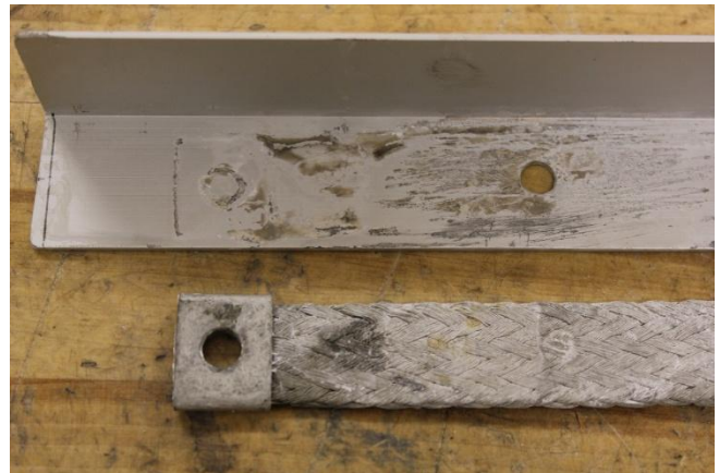
Fig. 7: Corrosion under alternate braid configuration
