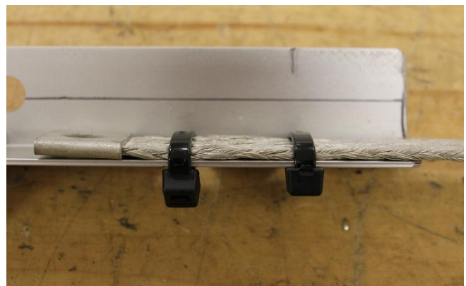
Fig. 3: Anodized aluminum angle with tin-plated copper braid
