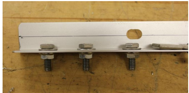
Fig. 1: Anodized aluminum angle with stainless hardware
