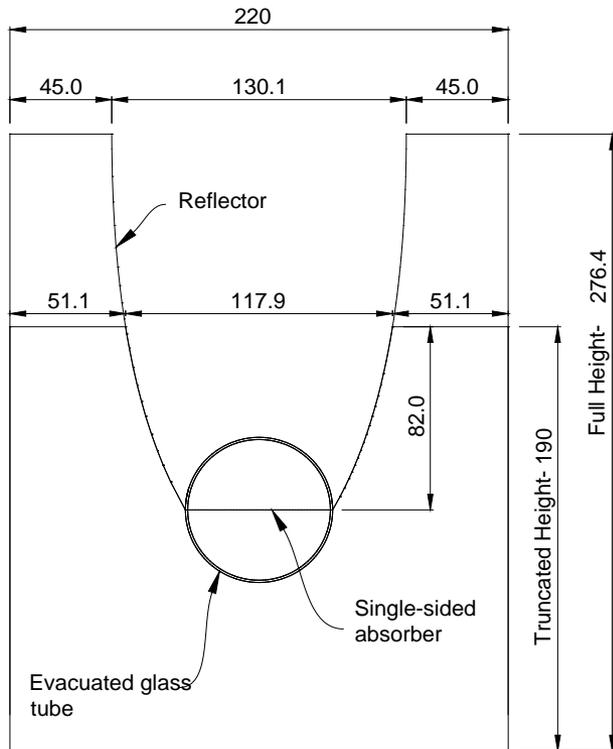
The fabricated full and truncated SSACPC solar collectors (dimensions in mm)
