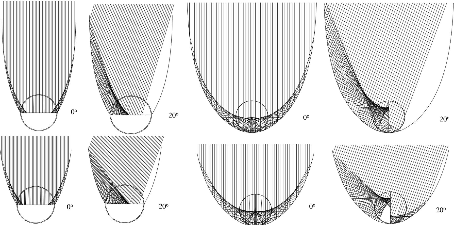
**Ray trace diagram-full and truncated SSACPC solar collectors at 0° and 20° incident angles**
