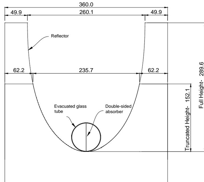
The fabricated full and truncated DSACPC solar collectors (dimensions in mm)
