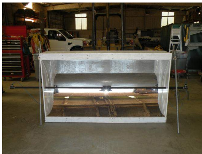
Fig 3: Final Parabolic Trough
