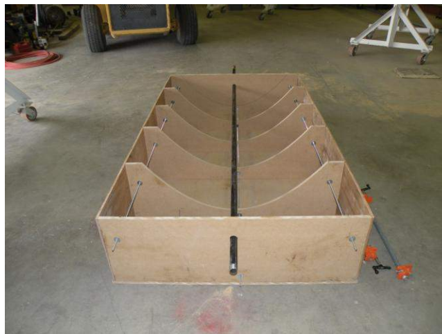
Fig 2: Parabolic trough showing the final shape of the parabola, absorber tube, and rebar for alignment.
