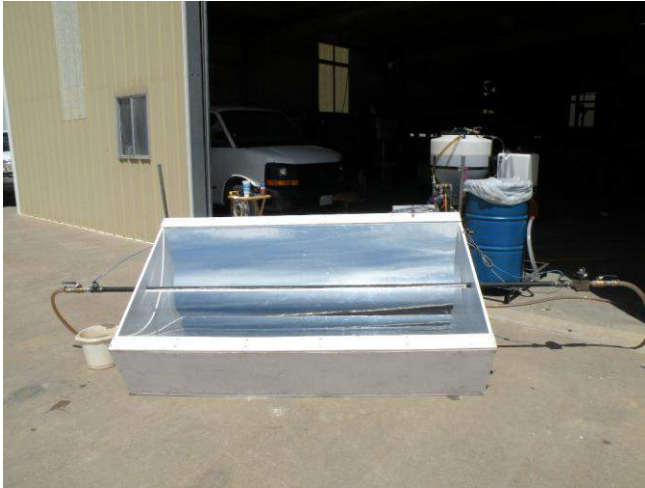
Fig 4: Parabolic trough being used for inline heat processing of biodiesel
