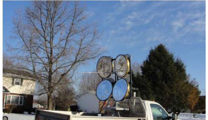
Figure 13 - 1/4 scale model mounted for high wind survival testing.
