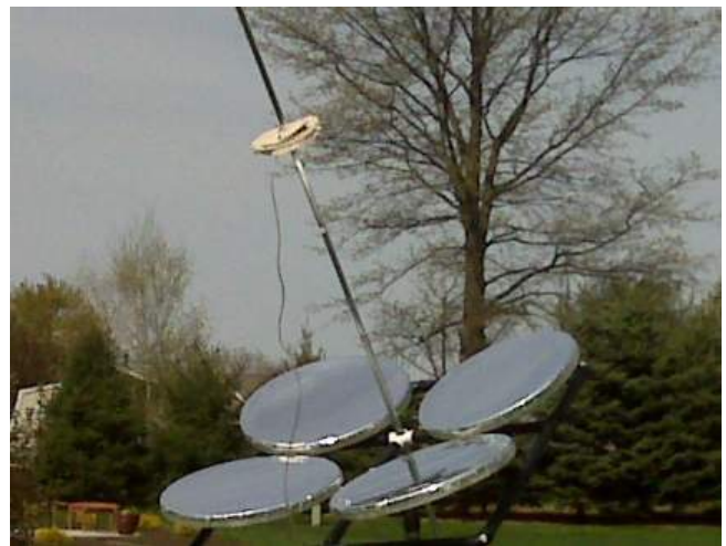
Figure 10- 4-dish tracking structure, configured as a dish/thermal system with integral receiver. (insulated receiver plate depicted.).
