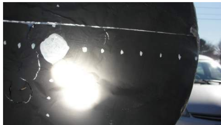
Figure 6- Characterized 4' dish at a 12' focal length.
