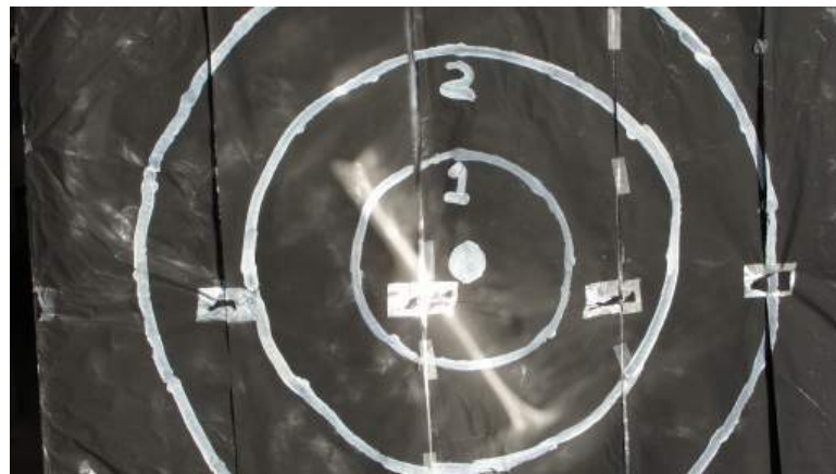
Figure 22- Off-axis by 45 degrees.. The focal spot becomes a focal line.
