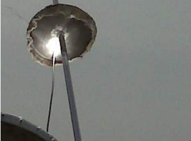
Figure 11- 4 dishes focused onto a thermocouple on insulated thermal receiver plate.
