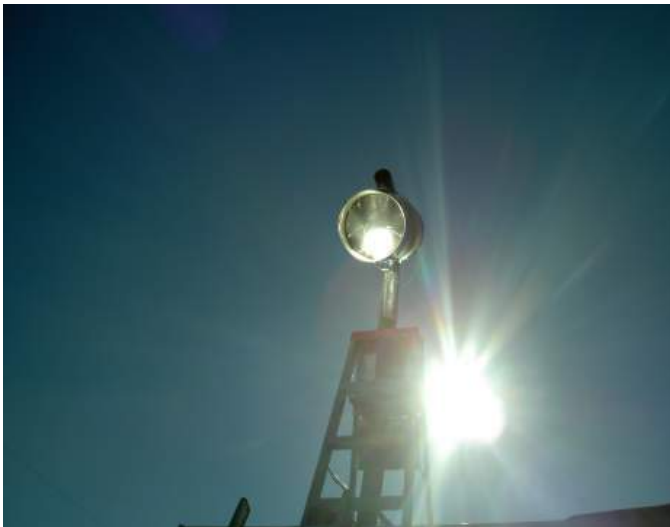
Figure 20- 8' diameter dish at 18' focal length
