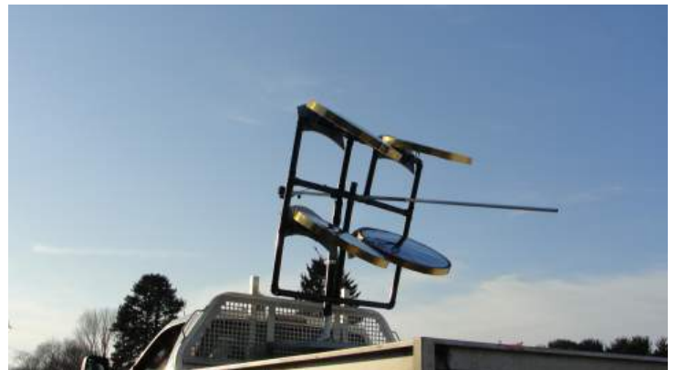
Figure 15 - Tracking structure at 50 mph. Note that film on the dishes are slightly pressurized to establish a safe convex shape, and also to prevent destructive rippling of the film.
