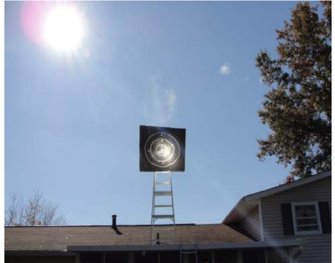
Figure 21- 8' diameter dish focal length adjusted to 37 feet, slightly off-axis to the sun.
