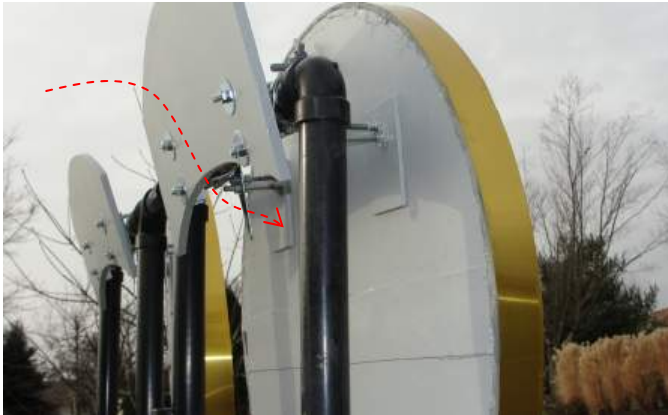
Figure 16- Wind deflector redirects oncoming wind downward, assisting upward rotation.
