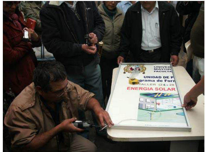
Fig 4 Pedro Sanchez installing the extruded aluminum frame on a 60 watt PV module in Peru. He used the vinyl poster announcing the PV course as the backing sheet.
