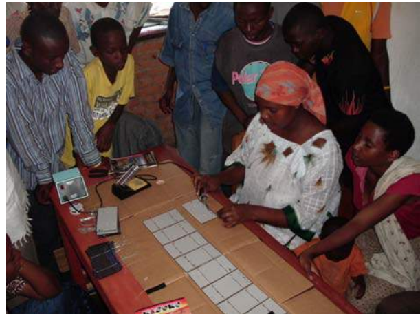
Fig 2 Soldering the PV cell strings in Rwanda, Africa
